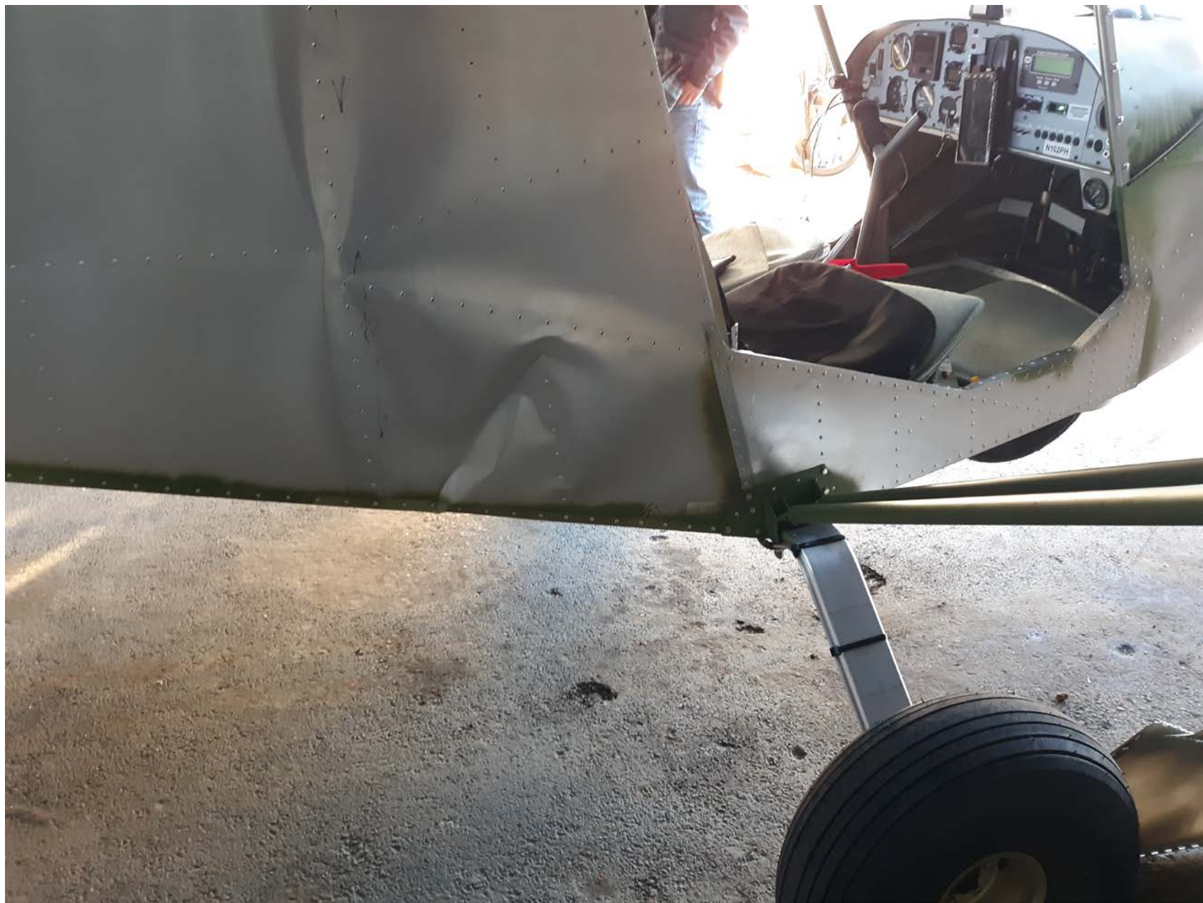
Photo 2 - View of fuselage damage (photo courtesy of unknown)
