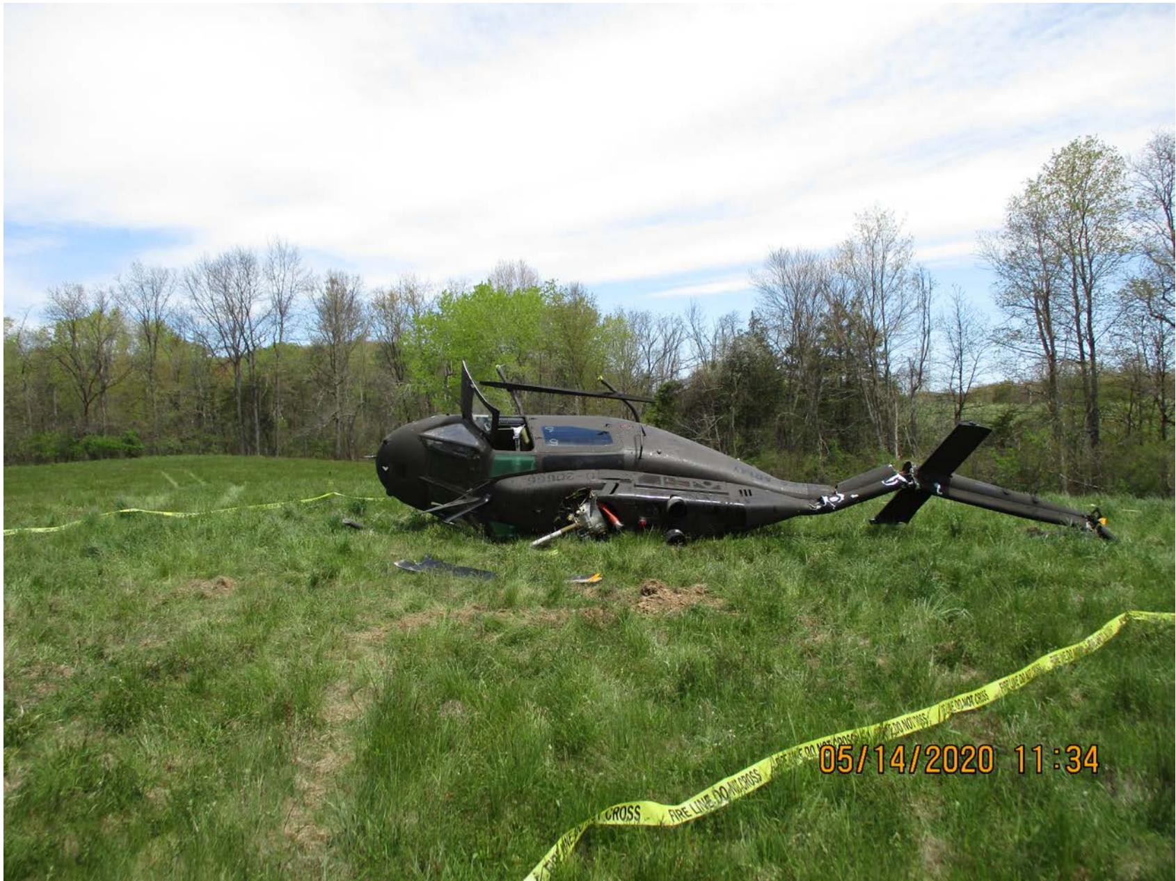
Photo 1 – View of tail-boom damage (photo courtesy of the FAA)
