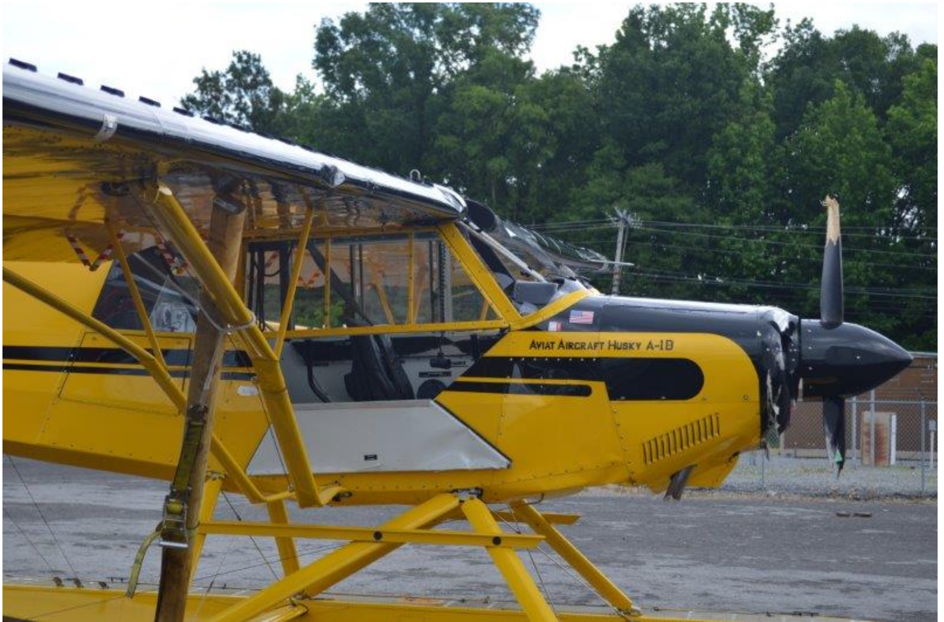
Photo 1 – View of the right-wing lift strut damage (photo courtesy of the pilot)
