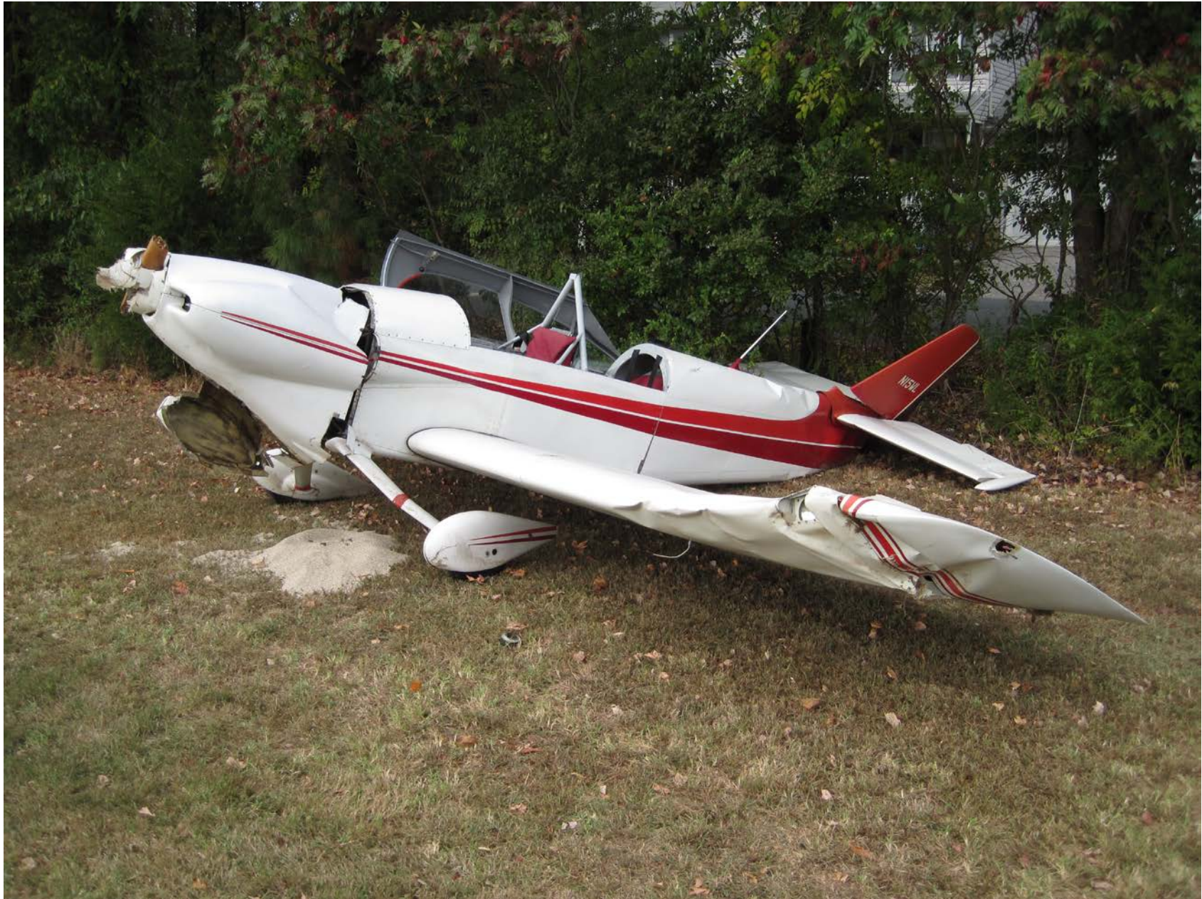
Photo 1 – View of fuselage and left wing damage (photo courtesy of the pilot)
