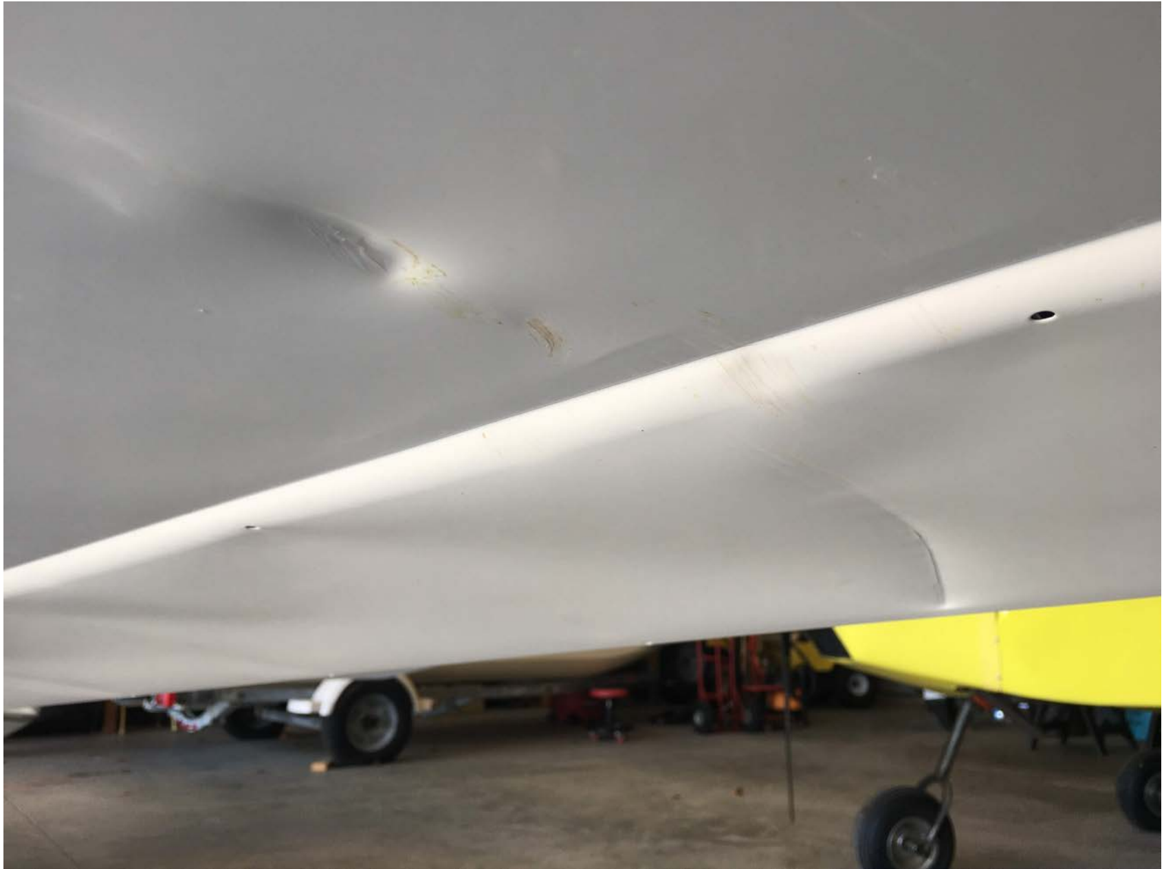
Photo 1 – View of left aileron damage (photo courtesy of pilot)
