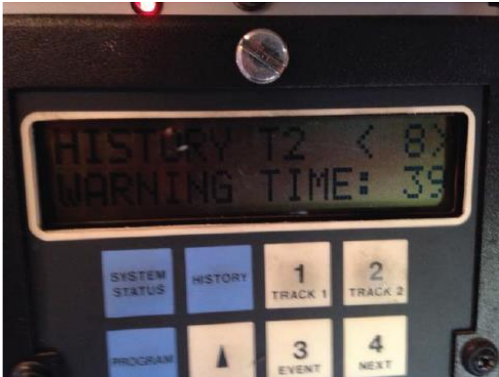
Figure-5 depicts warning time of the Grade Crossing Predictor to be 39 seconds
