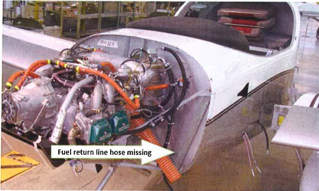
Figure 2 – Fuel system without the fuel return line
