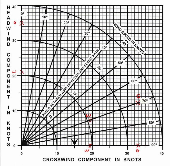
**INSTRUCTIONS:** Select the headwind component along the left side, and follow the curved line representing the headwind component until it intersects the angled straight line representing the degrees off the runway centerline the wind is coming from. Travel straight down to the bottom of the chart to find the crosswind component. In the example, there is a 30 knot headwind at a 30° angle to the runway, yielding a crosswind component of 15 knots – the legal maximum for CAP flight.
