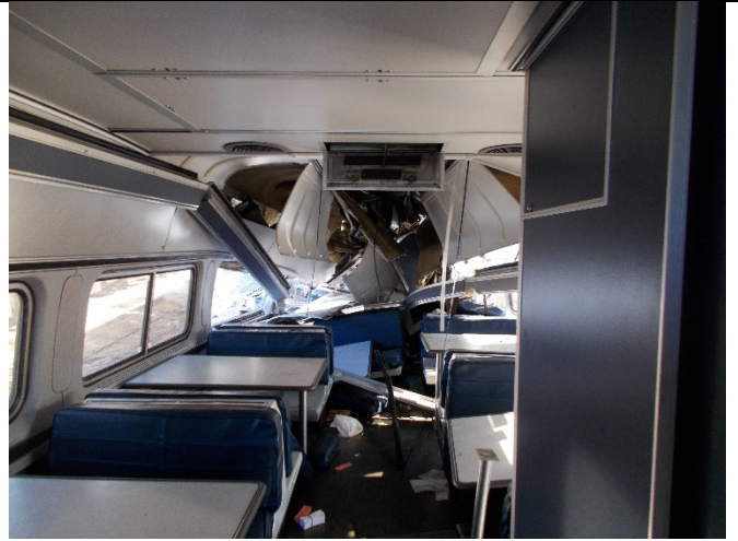
Figure 16- The rear section of car 28002 post recovery (Credit: FRA)
