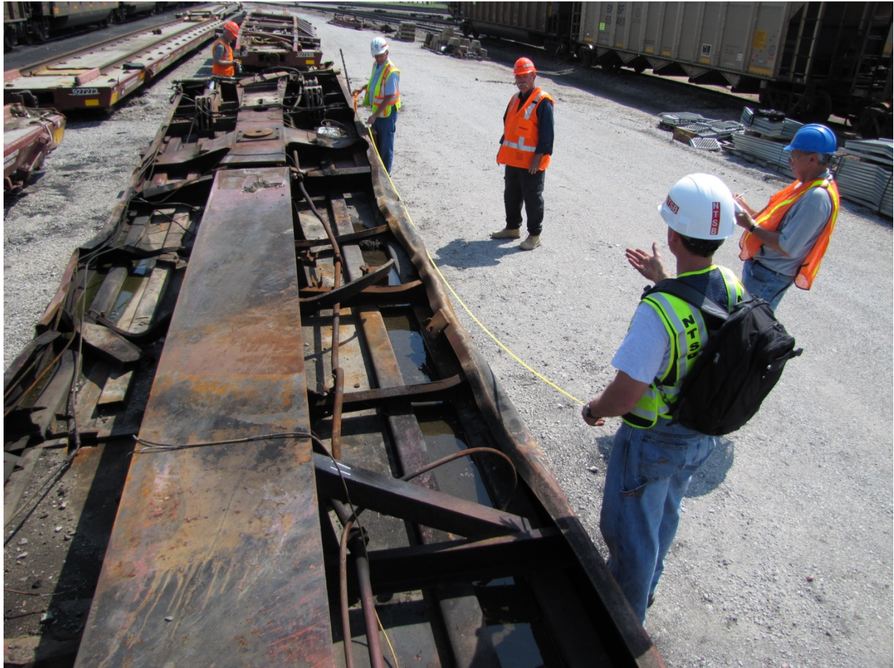
Exhibit 64-Photo Showing Damage to the Side Sill on BNSF 927022
