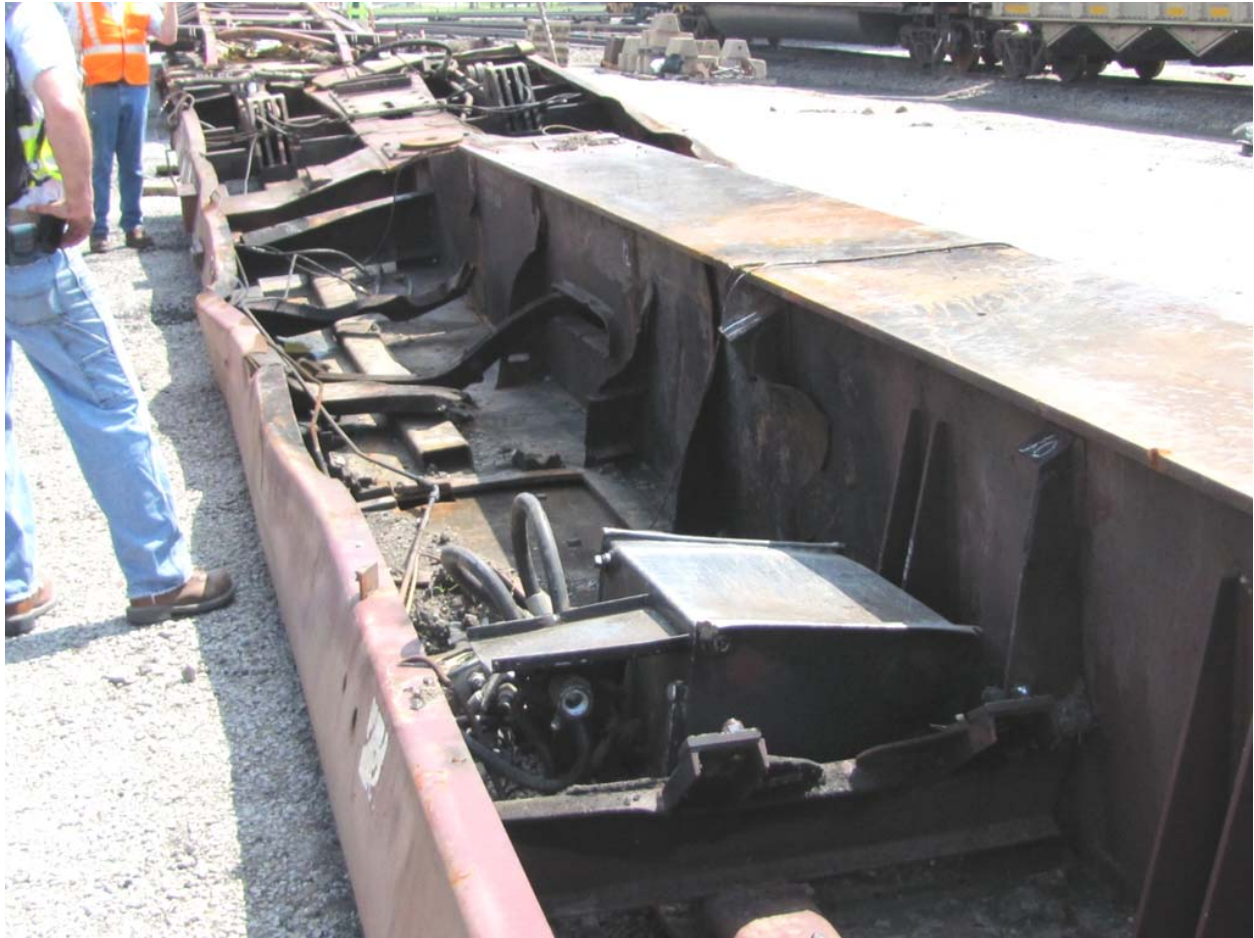
Exhibit 63-Photo Showing Damage to the Cross Bearers on BNSF 927022
