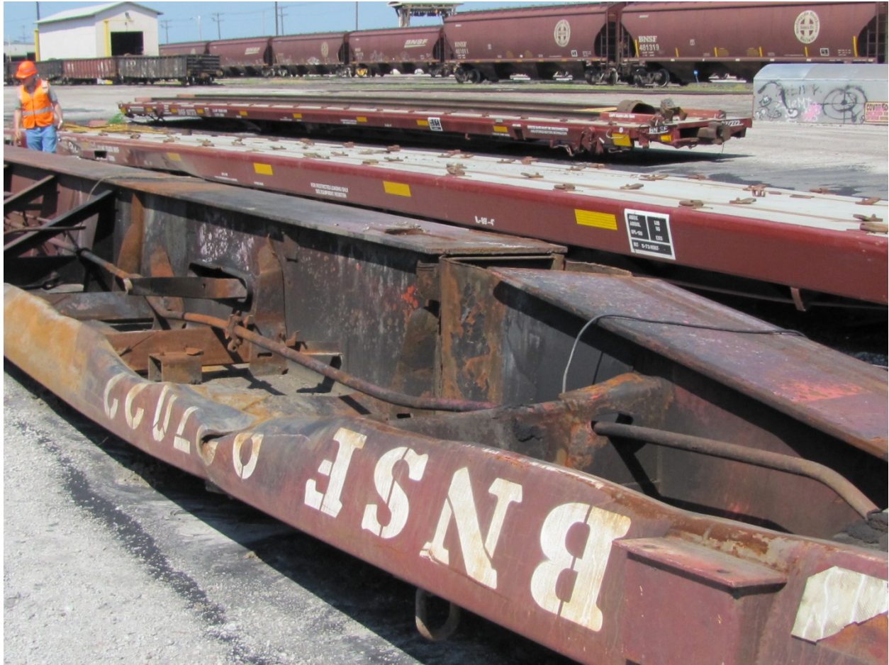
Exhibit 62-Photo Showing Damage to the Cross Bearers on BNSF 927022
