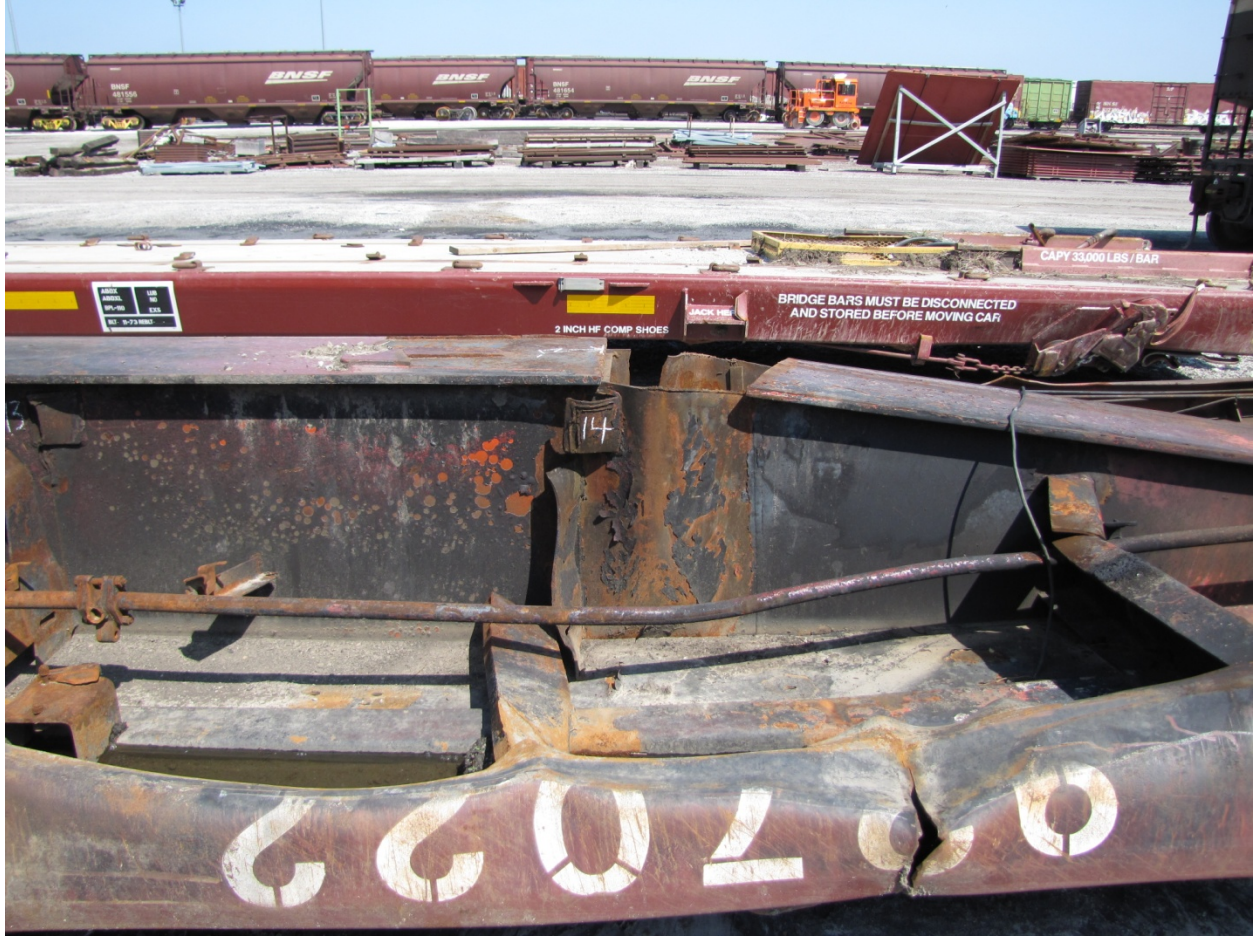
Exhibit 61-Photo Showing Mid-Section of the Centersill Damage on BNSF 927022
