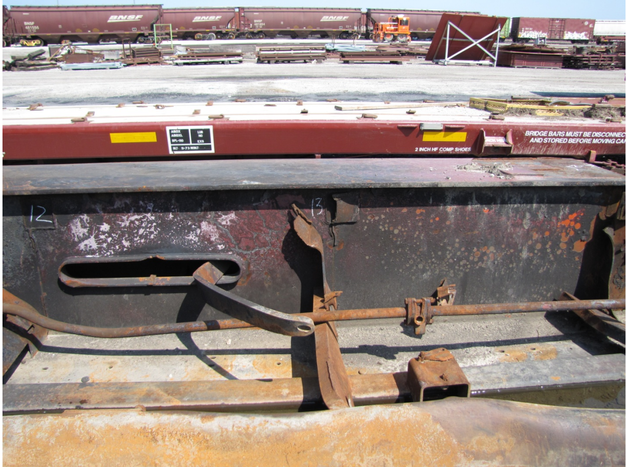
Exhibit 60-Photo Showing Mid-Section of the Centersill Damage on BNSF 927022
