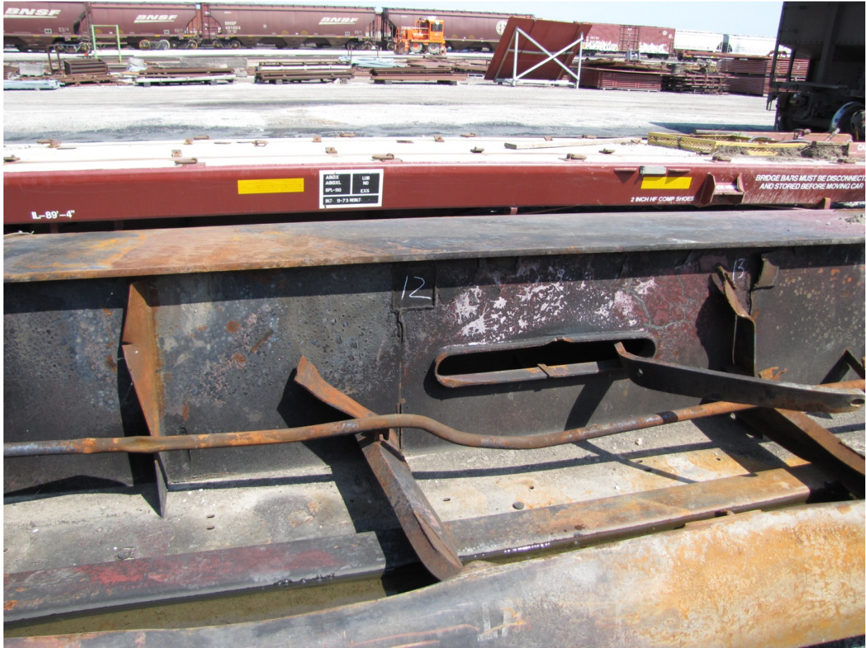
Exhibit 59-Photo Showing Mid-Section of the Centersill Damage on BNSF 927022
