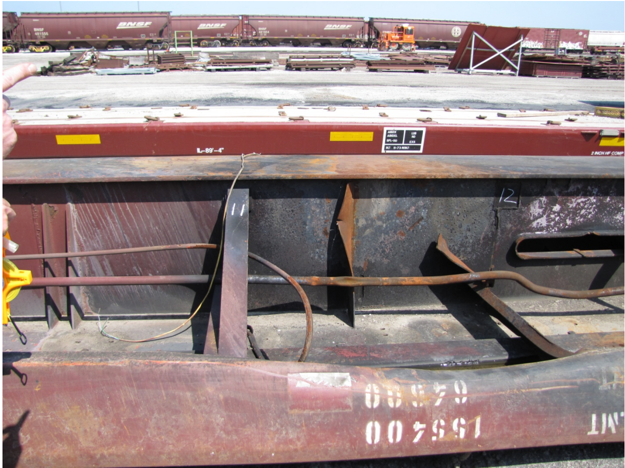
Exhibit 58-Photo Showing Mid-Section of the Centersill Damage on BNSF 927022
