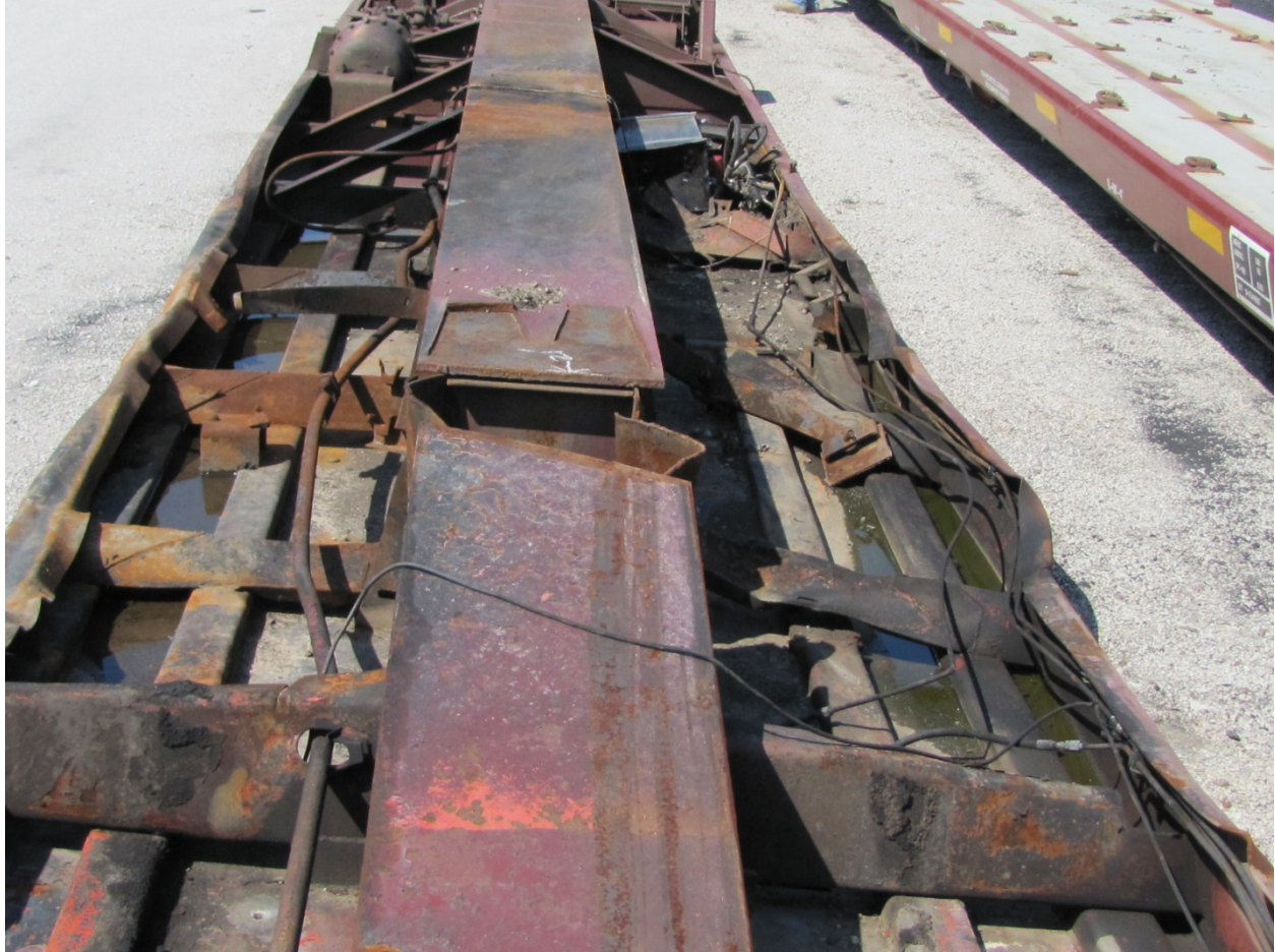
Exhibit 56-Photo Showing A-End of the Centersill Damage on BNSF 927022
