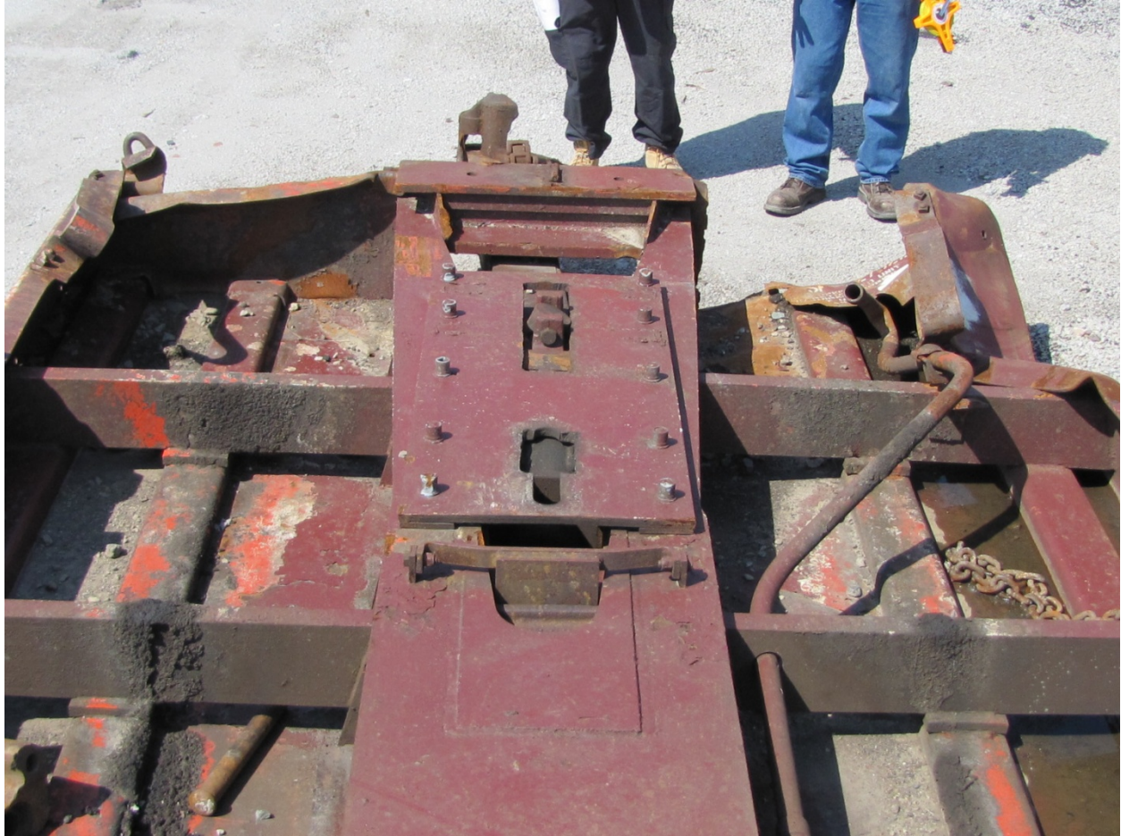
Exhibit 55-Photo Showing B-End Damage to BNSF 927022
