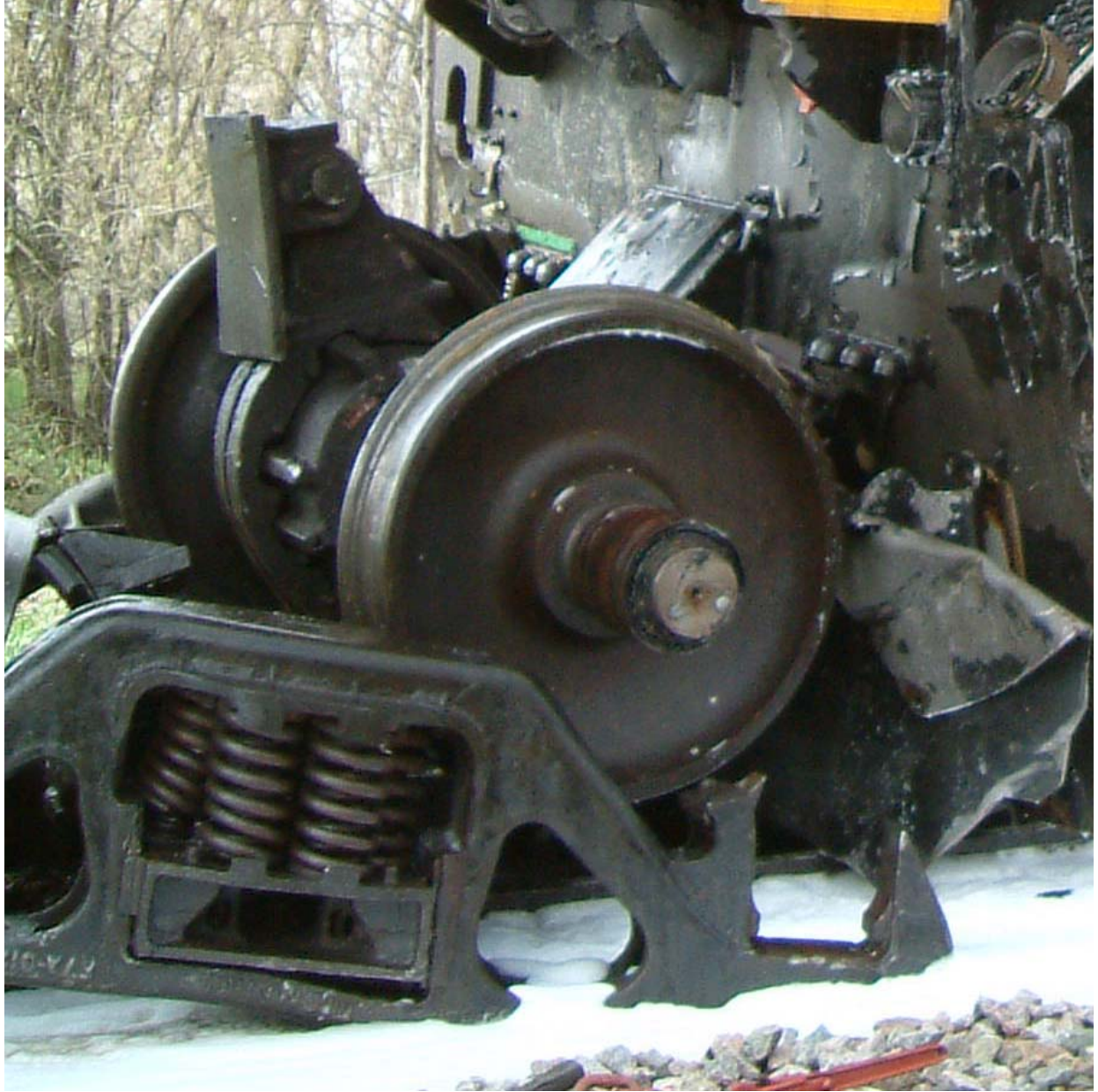
Exhibit 53-Photo Showing Powered Axle Assembly from HZGX-150 Clip Car in Front of BNSF 9159
