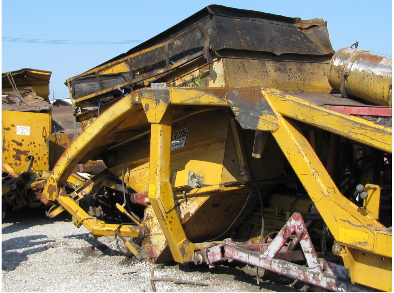
Exhibit 51-Photo Showing Damage to Saddle Assemblies on HZGX-150 Clip Car
