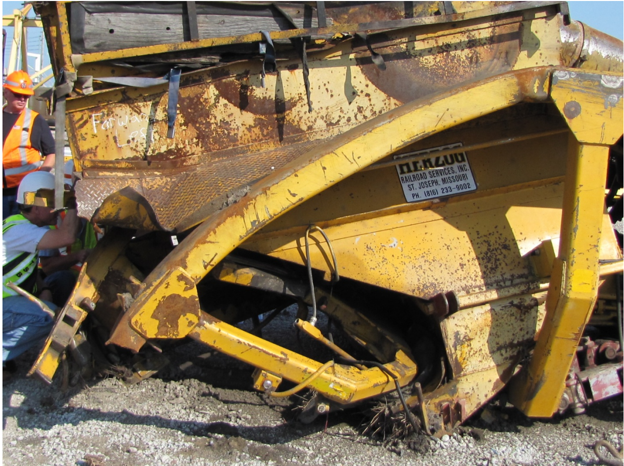
Exhibit 50-Photo Showing Bent Left Side 'Side Sill' on HZGX-150 Clip Car
