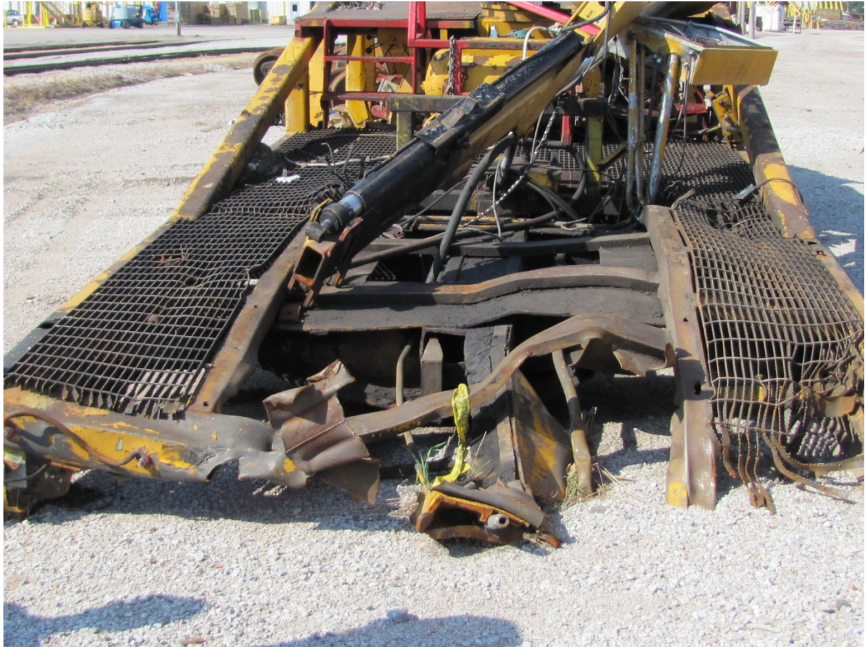
Exhibit 49- Photo Showing Rear End Section of Center Sill Crushed, Twisted and Buckled on HZGX-150 Clip Car
