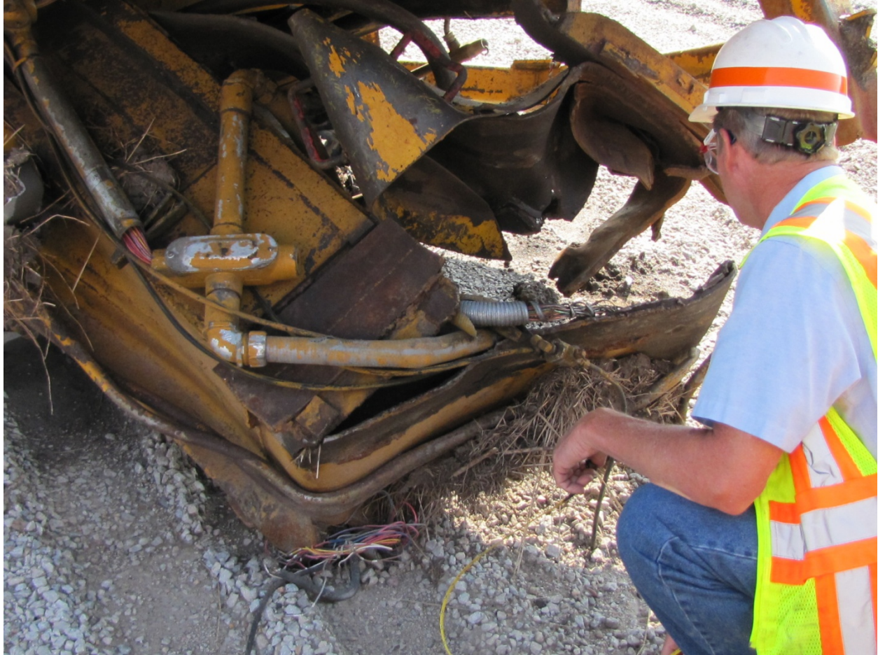
Exhibit 48-Photo Showing Rear Section of Center Sill Severed, Bent and Twisted on HZGX-150 Clip Car
