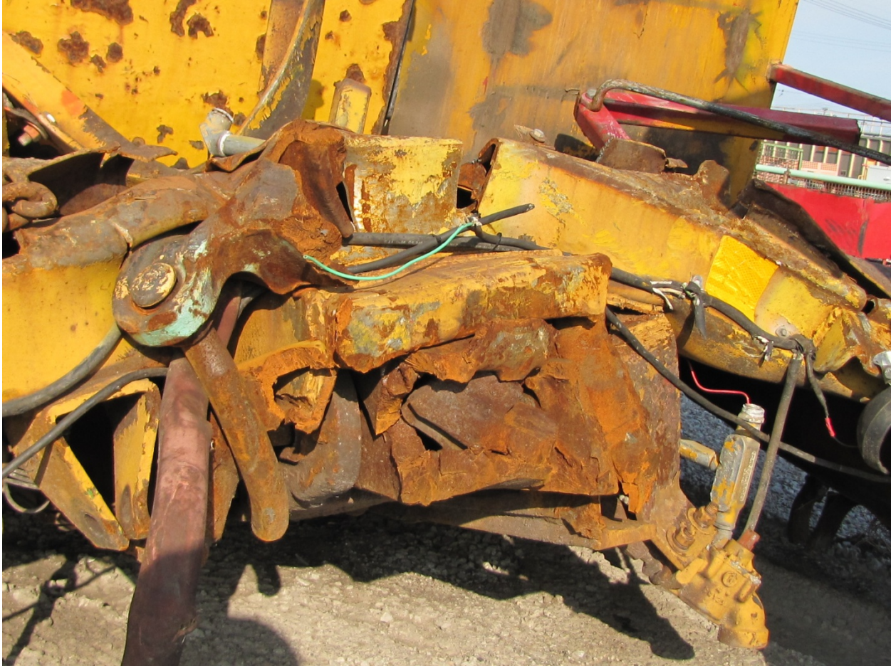
Exhibit 45-Photo Showing Damaged Draft Pocket of the Struck End on HZGX-150 Clip Car
