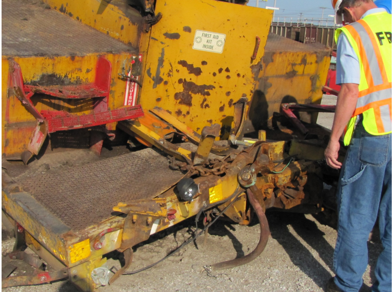
Exhibit 44-Photo Showing Damaged End Sill of the Struck End on HZGX-150 Clip Car
