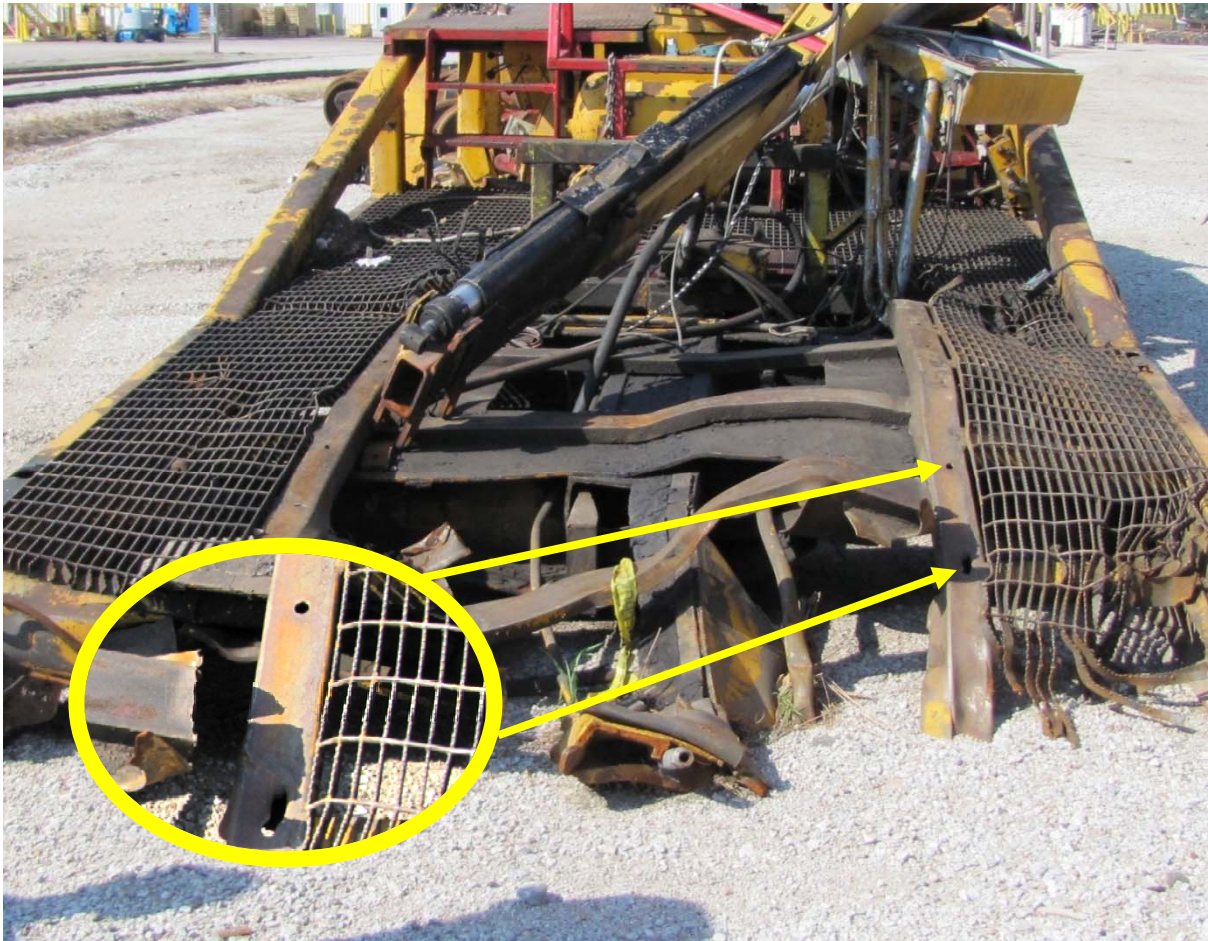
Exhibit 43-A- Photo Showing Condition of Select HZGX-150 Engine Mounting Points
