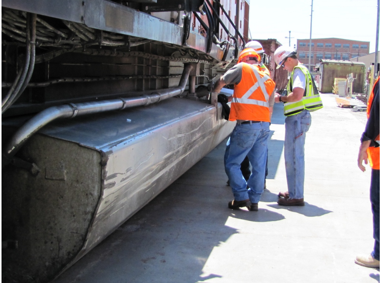
Exhibit 42-Photo Showing Damaged Fuel Tank of BNSF 9159
