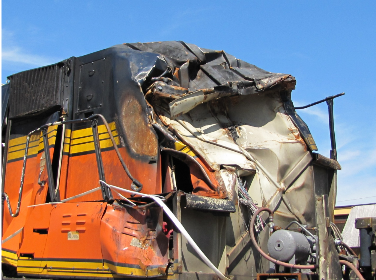
Exhibit 41-Photo Showing Damaged Electrical Locker Assembly of BNSF 9159
