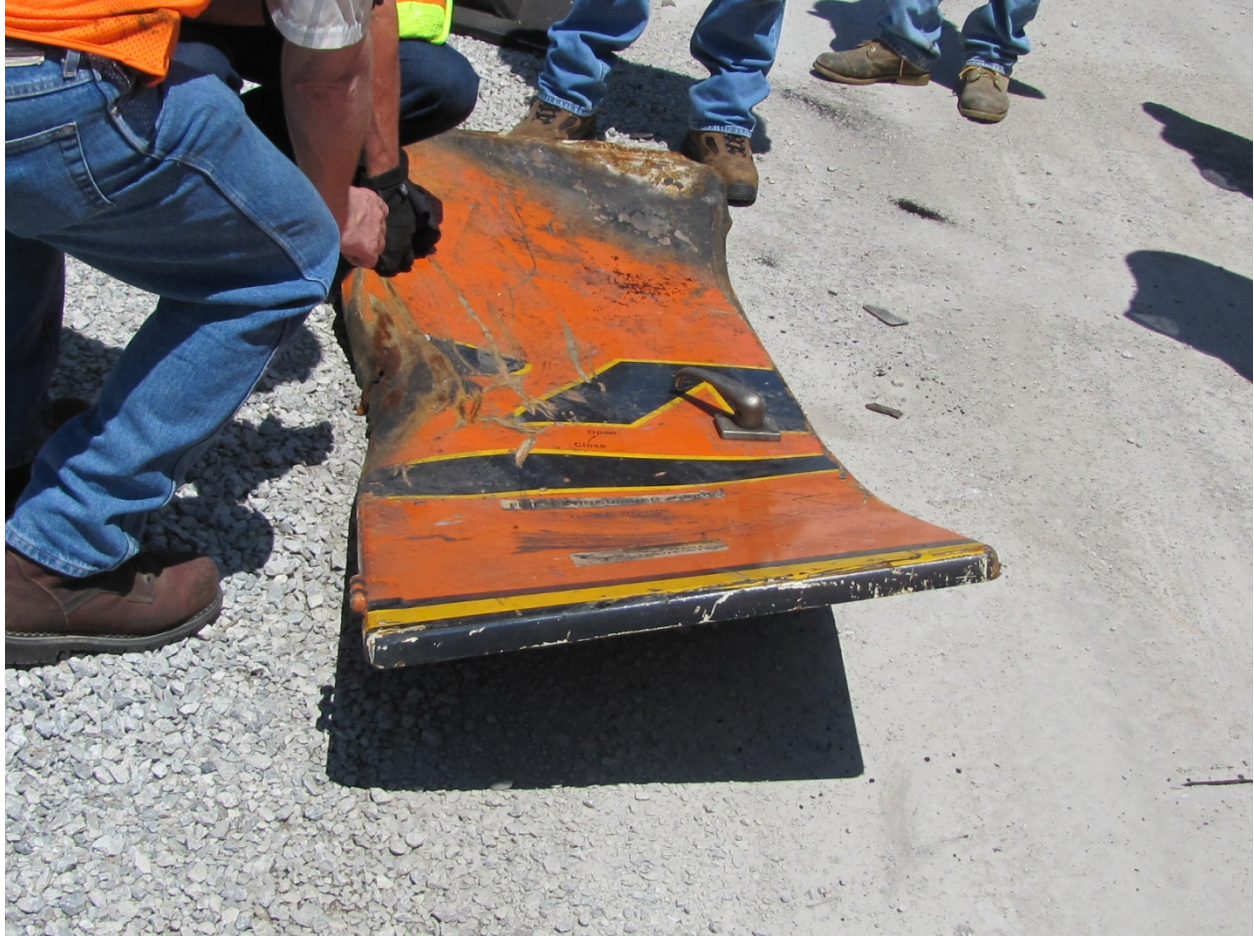
Exhibit 40-Photo Showing Damaged Door of BNSF 9159
