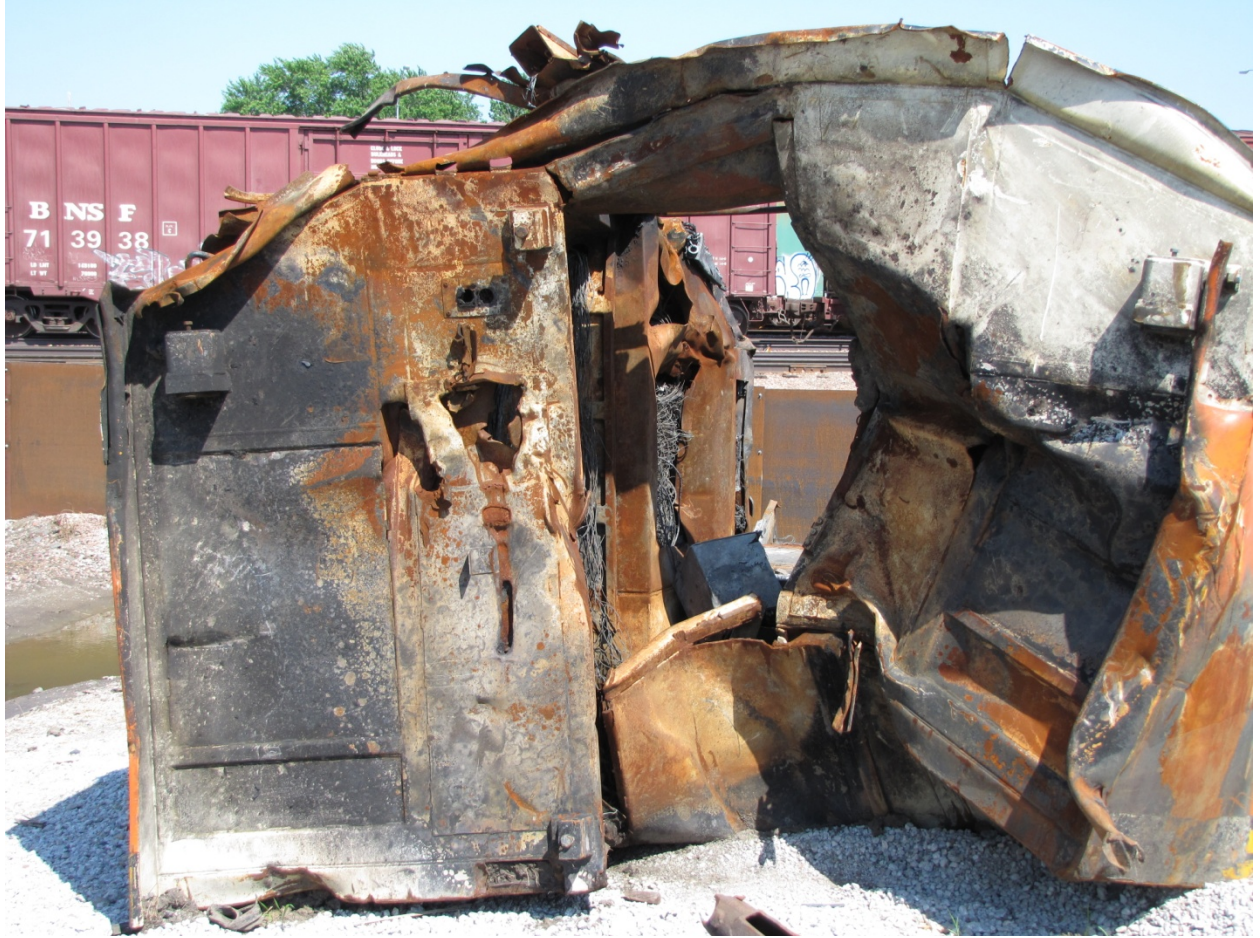
Exhibit 39-Photo Showing Damaged Inner Doorway of Operating Cab of BNSF 9159
