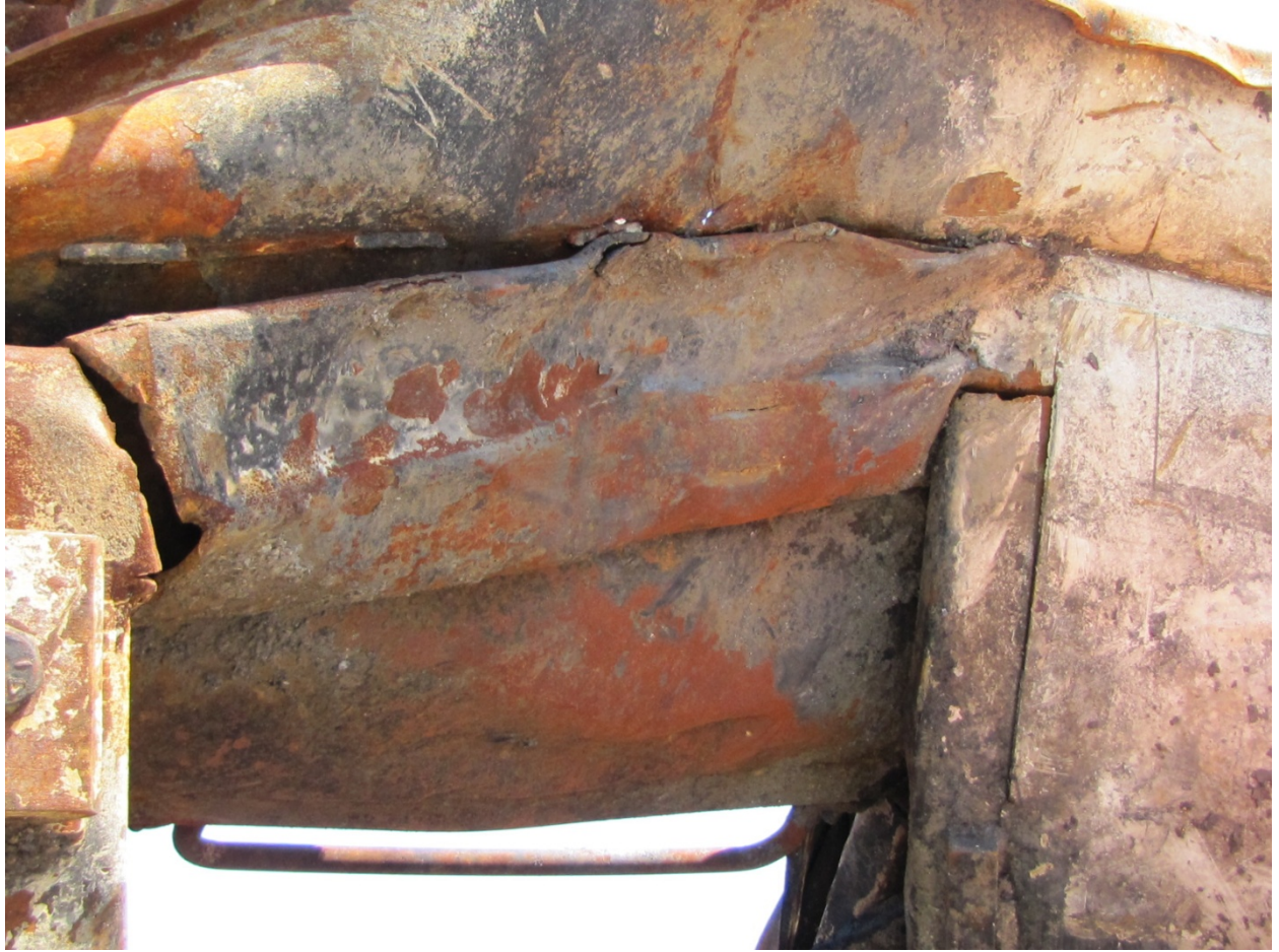
Exhibit 38-Photo Showing Damaged Upper Doorframe of Operating Cab of BNSF 9159
