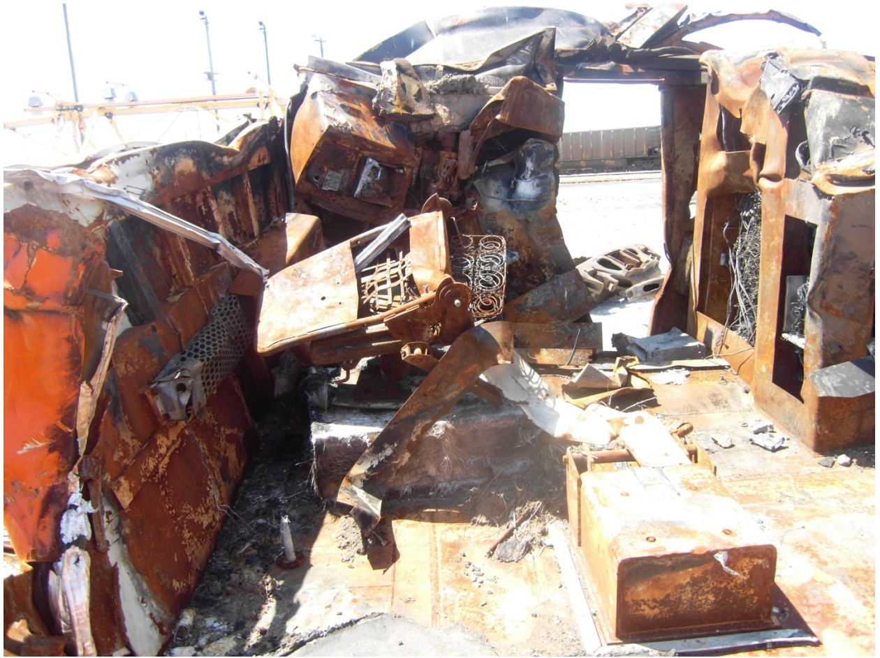
Exhibit 37-Photo Showing Damaged Left Side of Operating Cab of BNSF 9159
