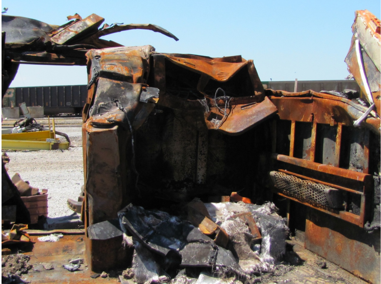
Exhibit 36-Photo Showing Damaged Right Side of Operating Cab of BNSF 9159
