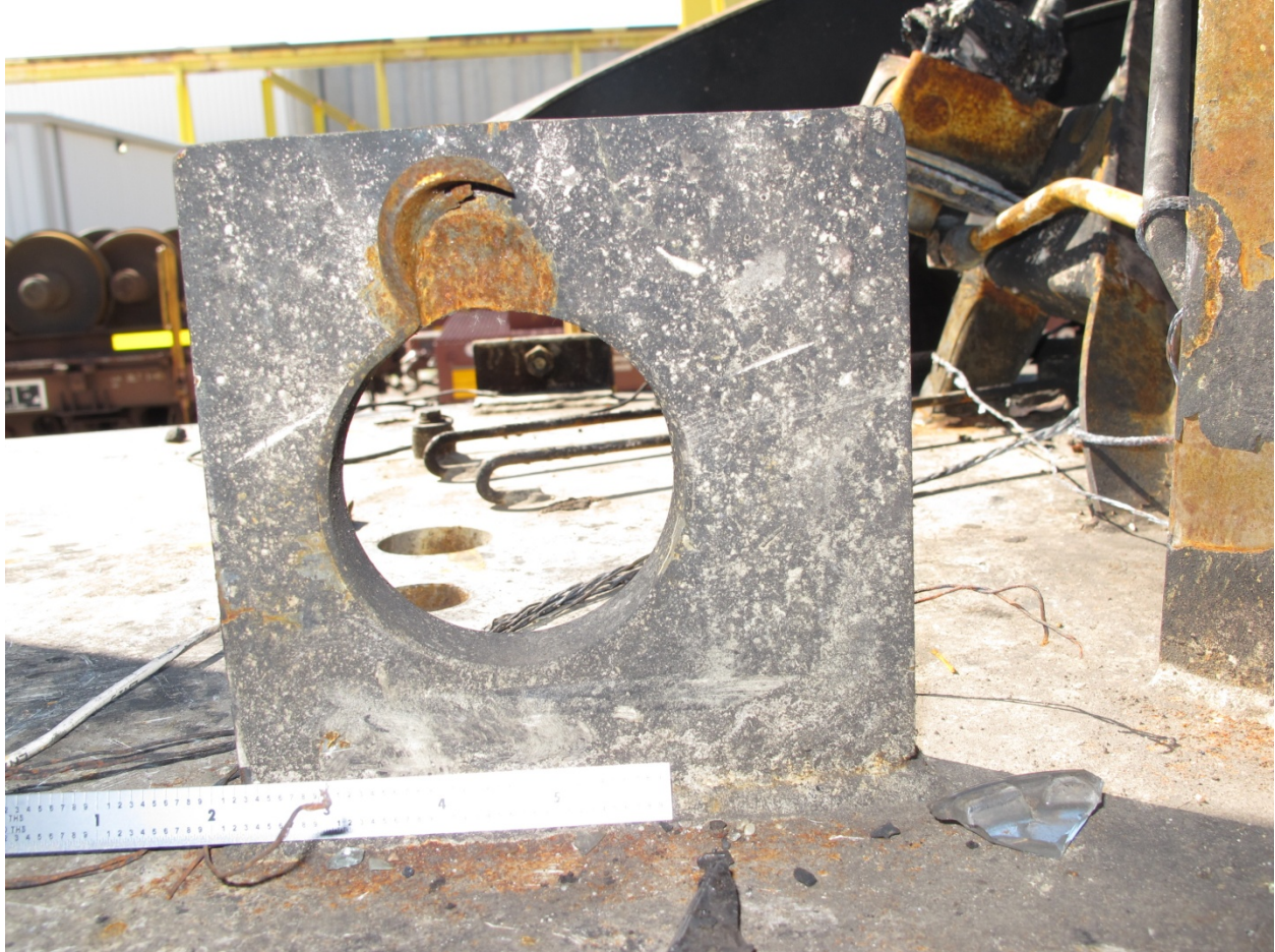
Exhibit 33-Photo Showing Forward Mounted Floor Bracket Damage on BNSF 9159
