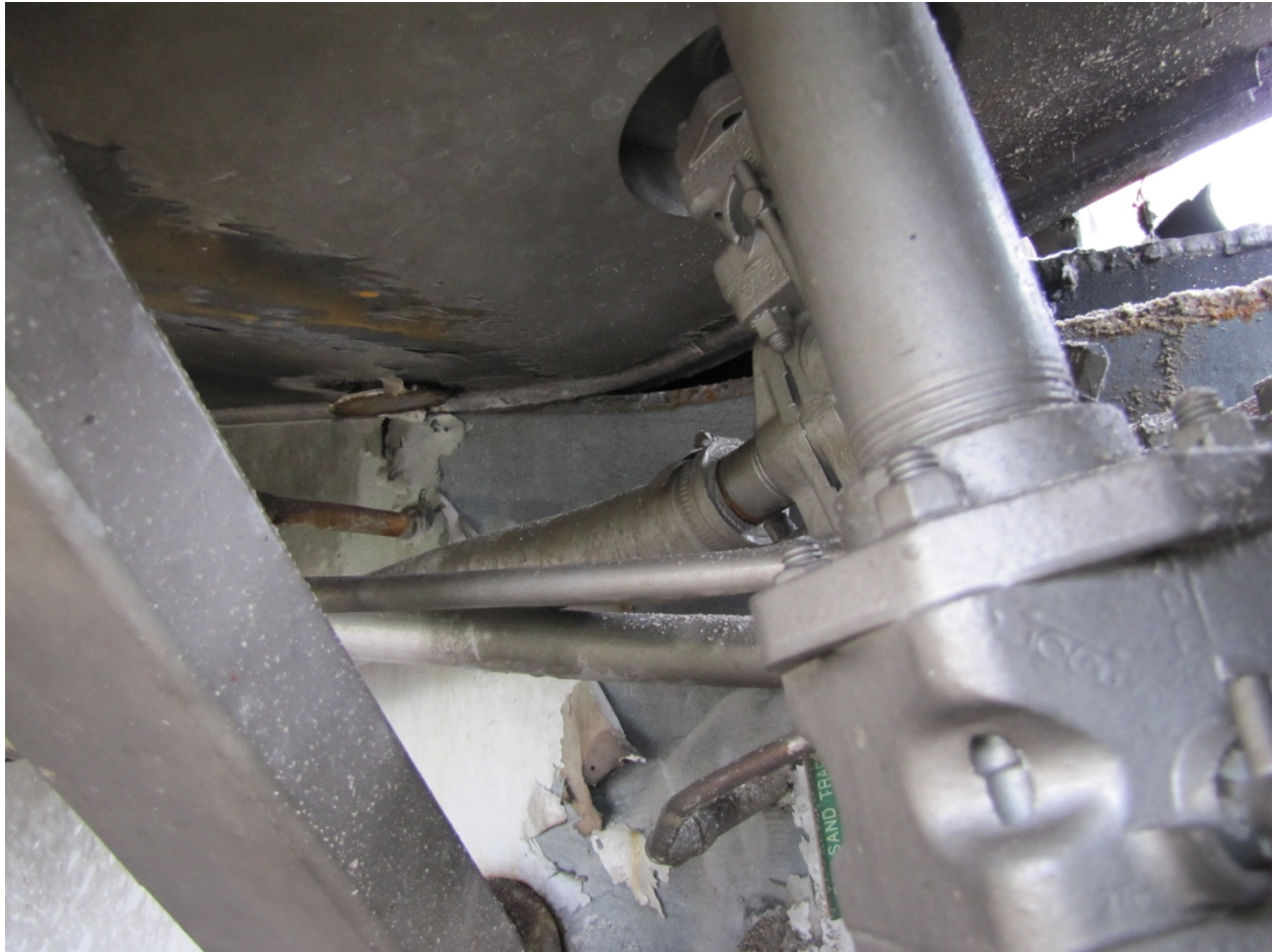
Exhibit 32-Photo Showing Left Side Centersill Separation from the Top Plate on BNSF 9159
