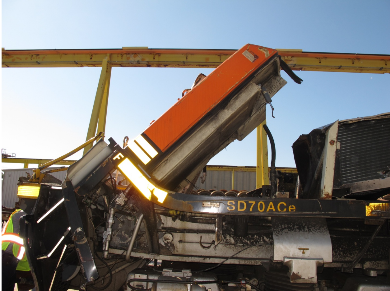
Exhibit 31-Photo Showing Centersill Deflection on BNSF 9159
