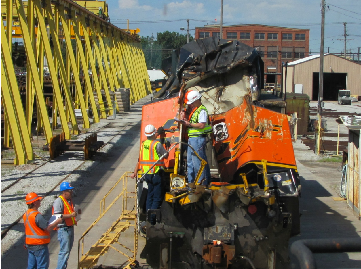
Exhibit 29- Photo Showing Left Side Shorthood Impact Damage of BNSF 9159
