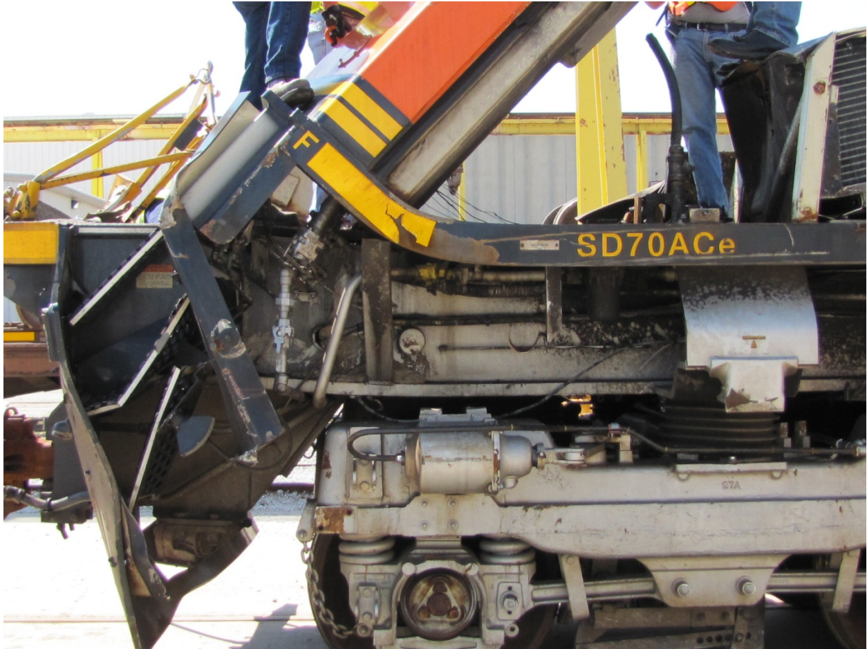
Exhibit 28-Photo Showing Left Side Shorthood Deflection of BNSF 9159
