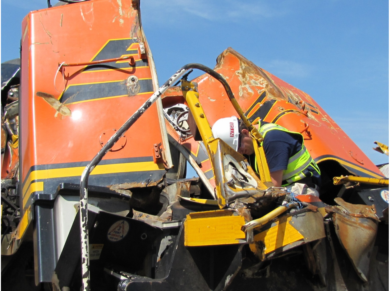
Exhibit 27-Photo Showing Right Side Short Hood Impact Damage of BNSF 9159
