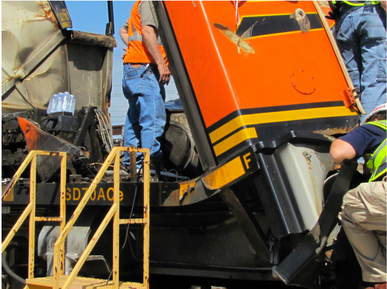
Exhibit 26-Photo Showing Right Side Shorthood Deflection of BNSF 9159
