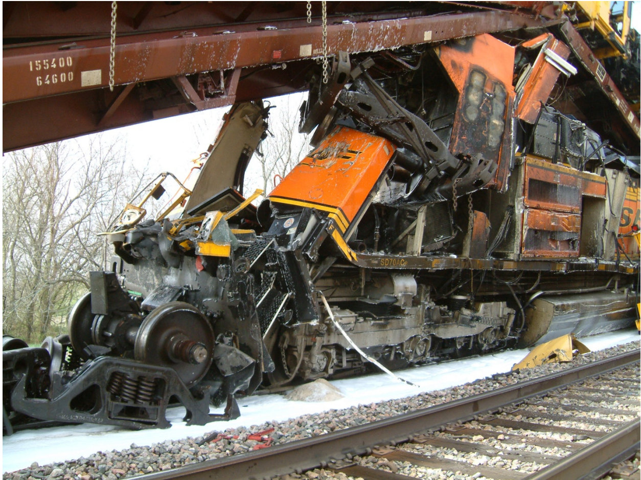
Exhibit 25-Photo Showing Damage to Shorthood and Separation of Doorframe (Door Laying on Top of Deck) BNSF 9159
