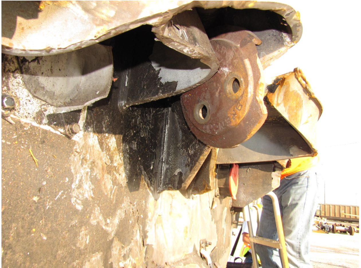
Exhibit 24-Photo Showing Right Side Damage to Anti-Climber Assembly of BNSF 9159
