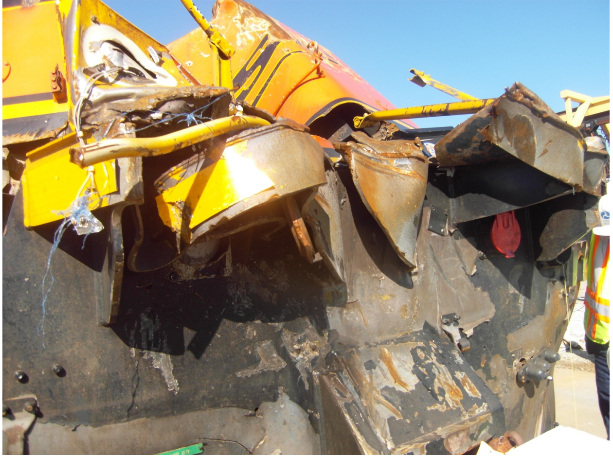
Exhibit 23-A-Photo Showing the General Condition of Damaged Anti-Climber of BNSF 9159
