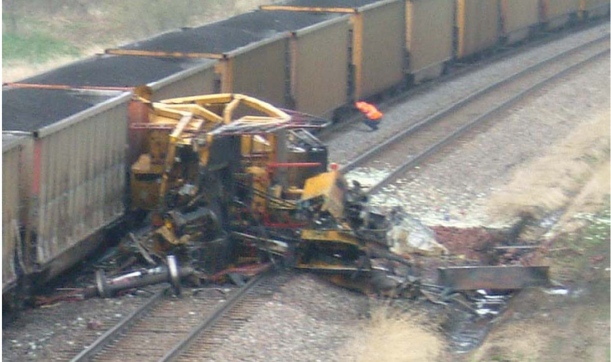
Exhibit 9-Photo Showing HZGX-150, Post Collision, on the North Side of Main Track Number Two
