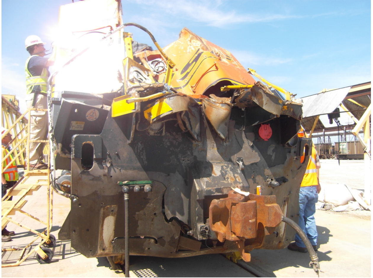
Exhibit 22-Photo Showing Damage to the End Plate on BNSF 9159
