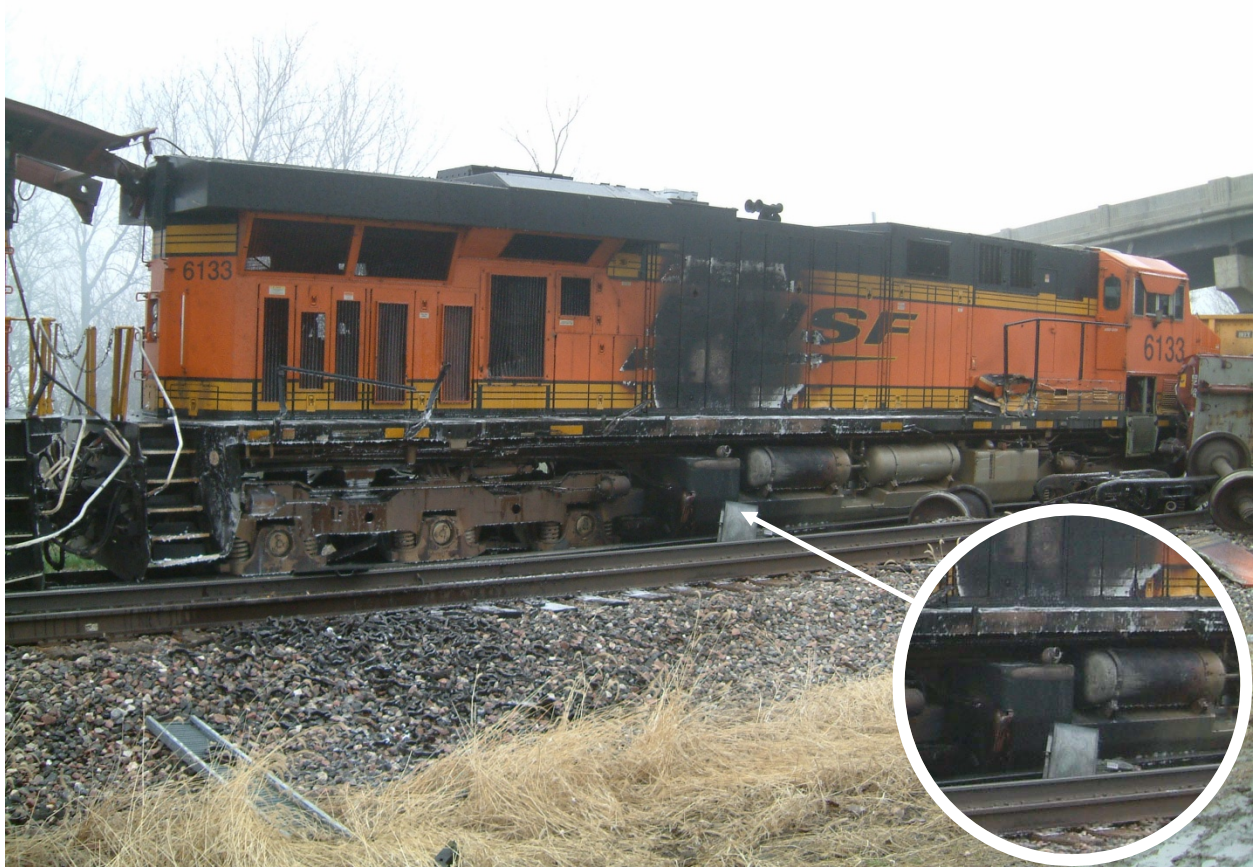
Exhibit 21-A-Photo Showing Compromised Fuel Tank on BNSF 6133
