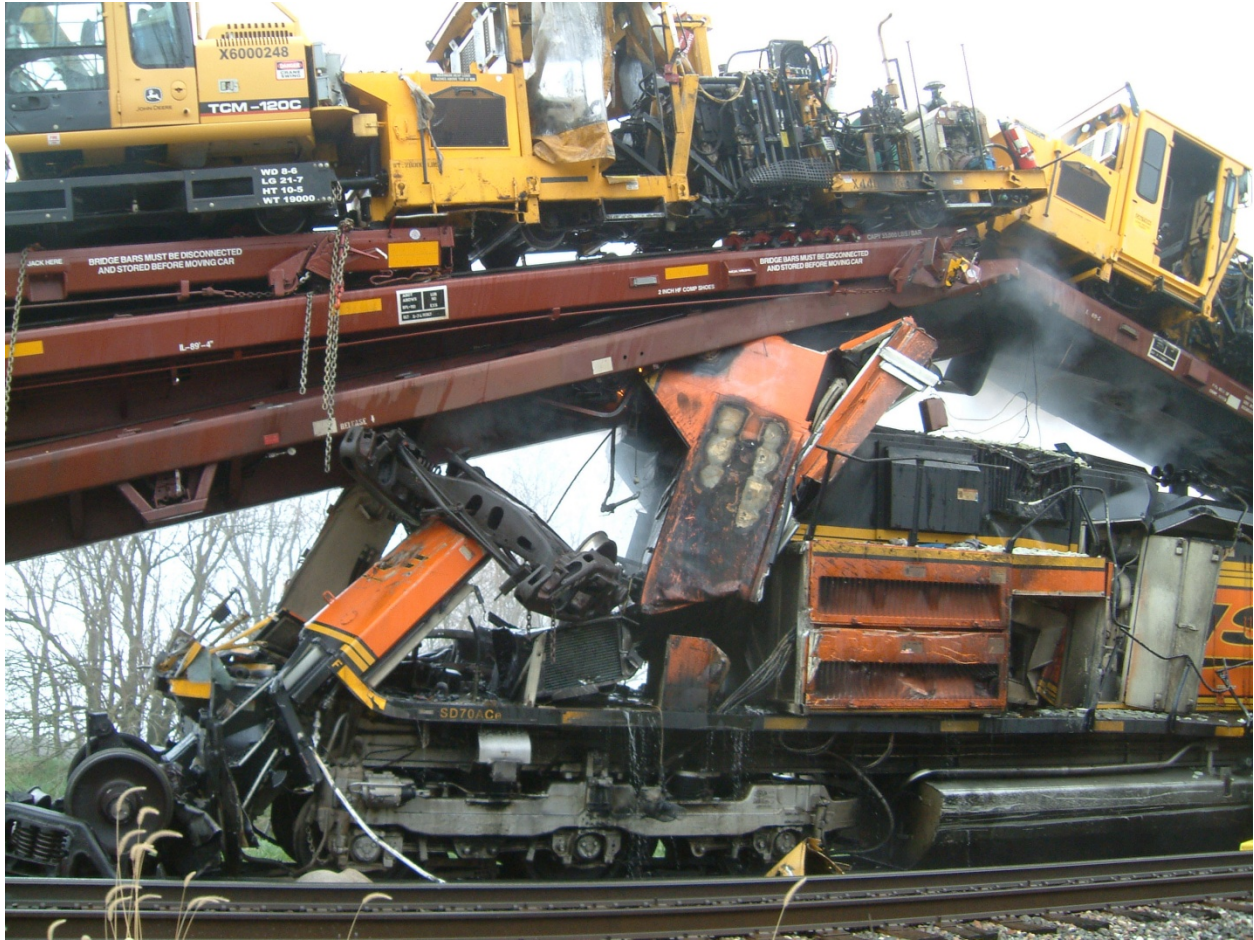
Exhibit 21-Photo Showing Short Hood Deflection and Cab Assembly Separation of BNSF 9159
