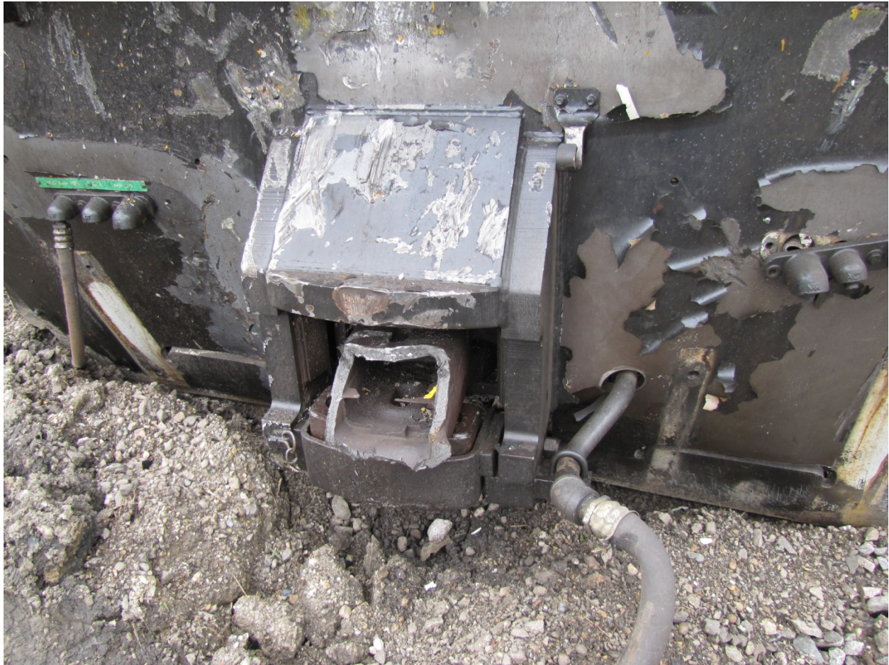
Exhibit 20-Photo Showing Sheared Coupler Assembly on Locomotive 9159
