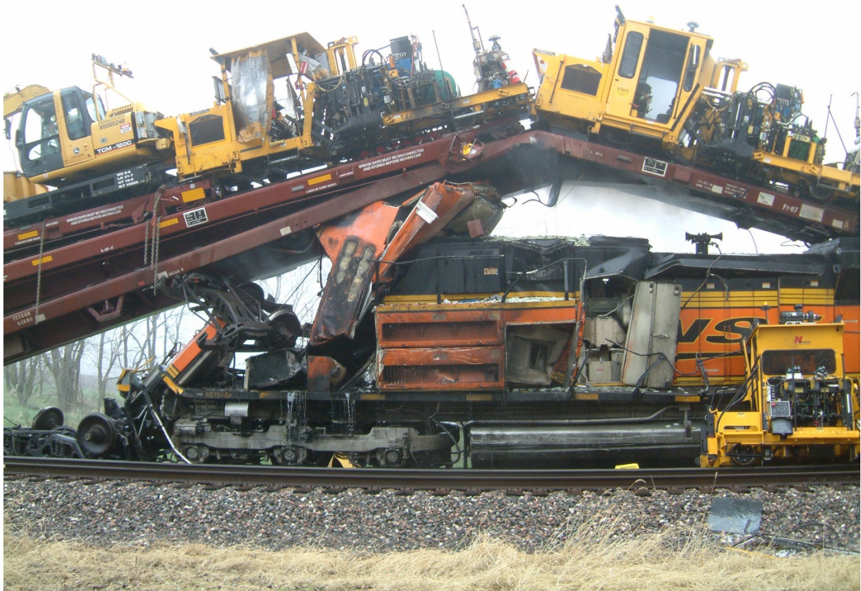
Exhibit 19-Photo Showing Compromised Front End on Locomotive BNSF 9159
