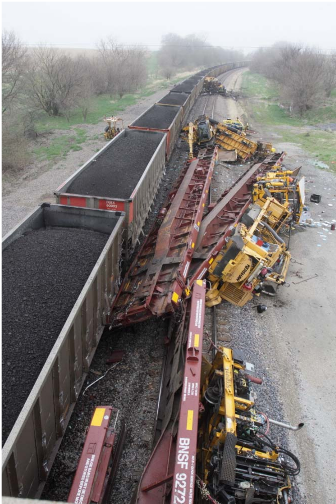
Exhibit 14- Photo Showing Lines 32-29 Lying on Their Side on the North Side of Main Track Number Two
